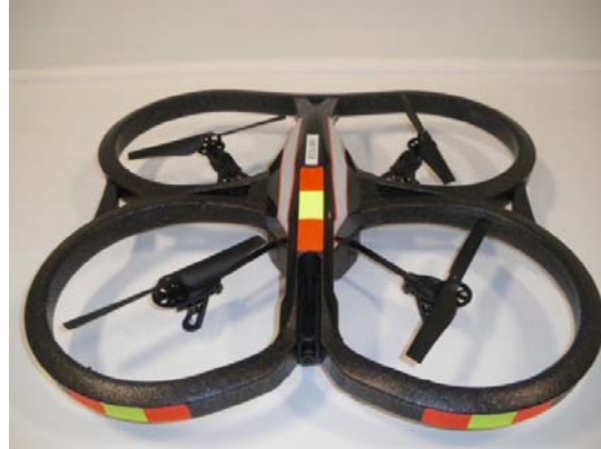
Figure 1: The Parrot AR Drone used in the tests.
