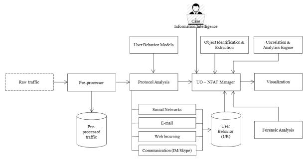
Figure 7: User-Oriented Network Forensic Analyser Design
