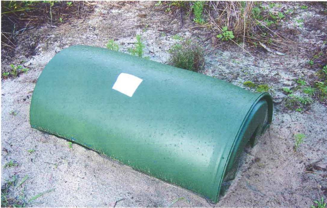
Plate 4.1 A 200L plastic drum cut in half lengthwise was used for the 'drum' bait station design (Photo: Malin Kordes, 2004).
