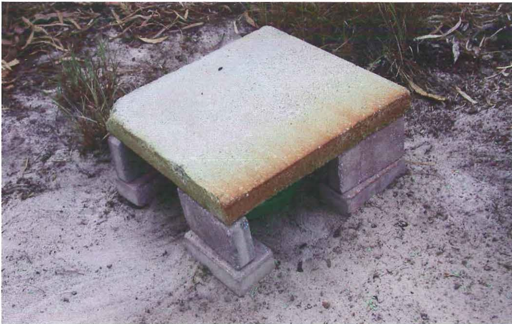
Plate 4.2 A 60 x 60 cm concrete slab supported on bricks was used for the 'slab' bait station design (Photo: Malin Kordes, 2004).
