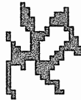
Figure 16. For the original image X depicted in Figure 15, \phi(X) = (X \cup \psi(X))^m is a closing for m=3 .
