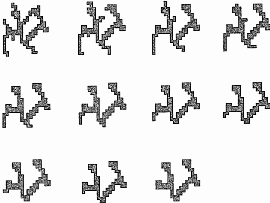
Figure 15. From left to right, top to bottom: original image X , (X \cap \psi(X)) , (X \cap \psi(X))^2, \dots, (X \cap \psi(X))^{10} , where \psi is the 4-median filter. In this case, \gamma(X) = (X \cap \psi(X))^n is an opening for n=10 (i.e. sequence converges after 10 iterations).
