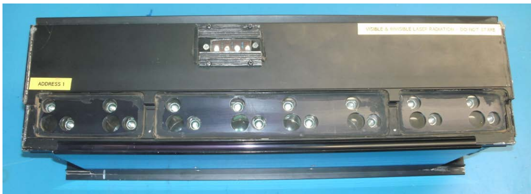
Figure 1.1. Prototype weed sensor developed by Photonic Detection Systems with 8 modules consisting of two lasers and a photodiode.
