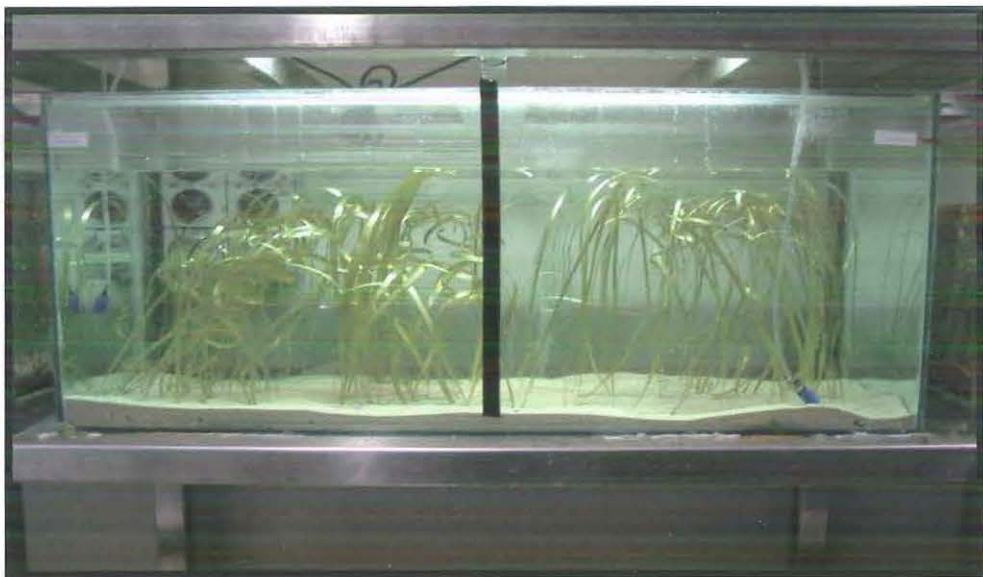
Plate 2.5 One of the three experimental aquaria; complete with Posidonia sinuosa (left) and Posidonia coriacea (right) artificial seagrass, used in the laboratory experiments to examine habitat preference of an abundant seagrass fish species.
