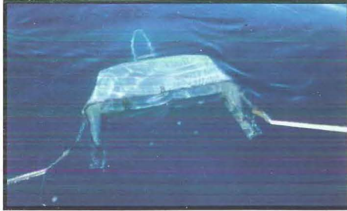
Plate 2.2 The beam trawl used to collect fish samples from each of the three seagrass habitats (G. Hyndes).
