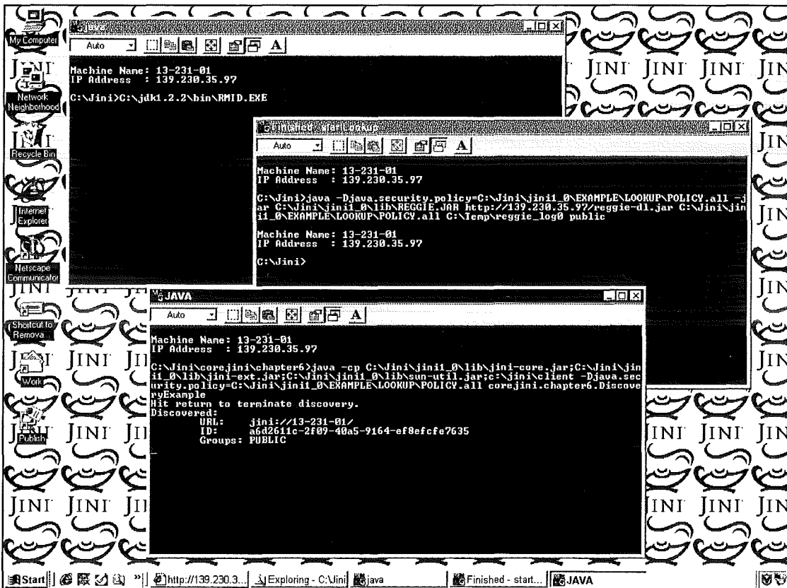
Figure 1 – The first lookup service is already running and consequently discovered by the discovering service entity.
