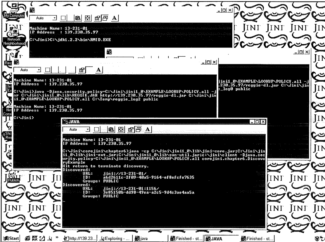
Figure 4 – The second lookup service is run and consequently discovered too by the discovering service entity.
