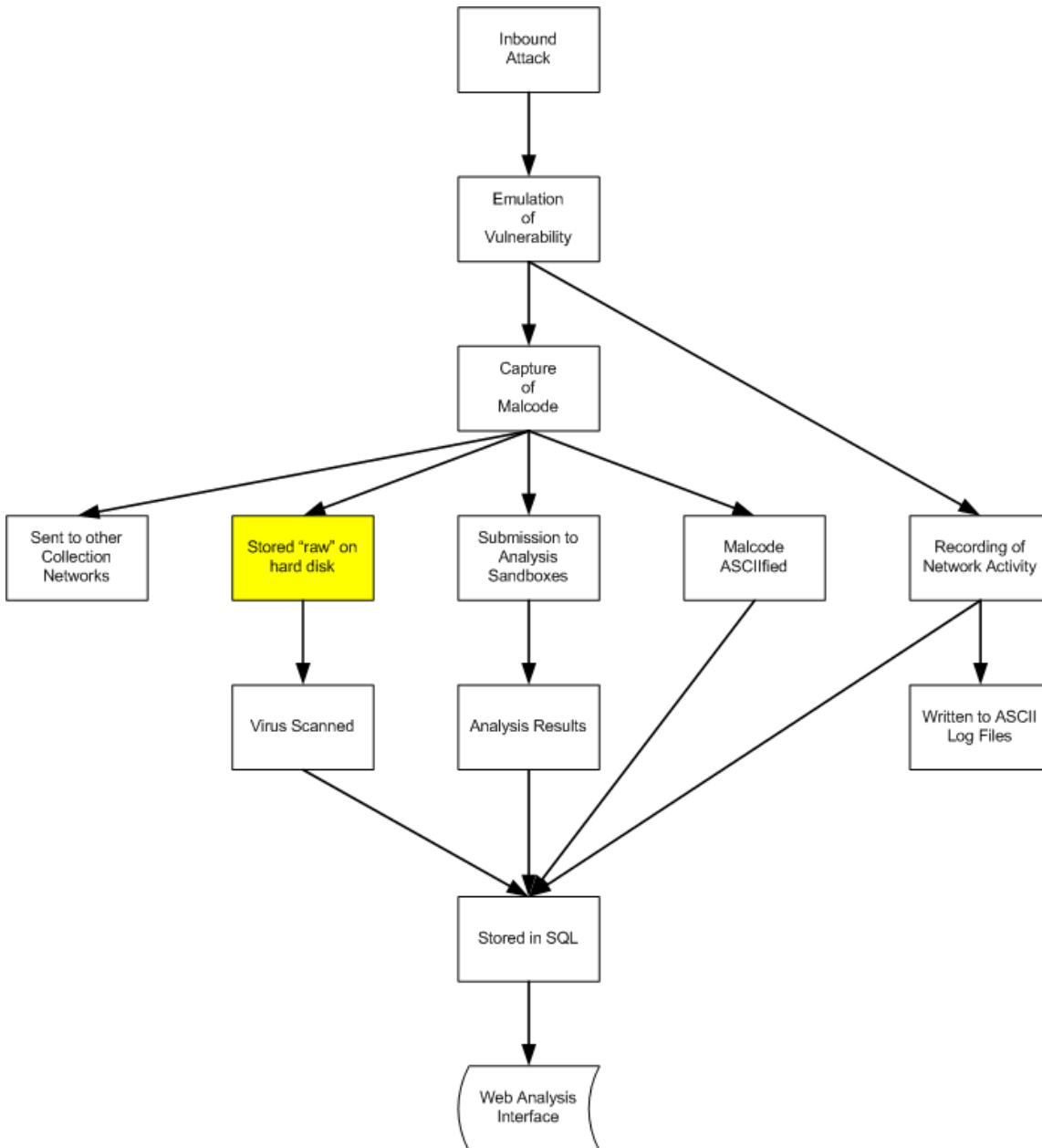
Figure 3-2 Model of the nepenthes malware collection system depicting the source (highlighted) of malware collected for this research.
