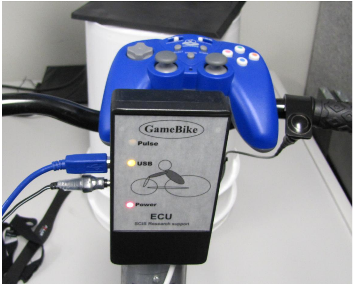
Figure 23 Close up of Heart Rate sensor box front mounted on bike handlebars.
