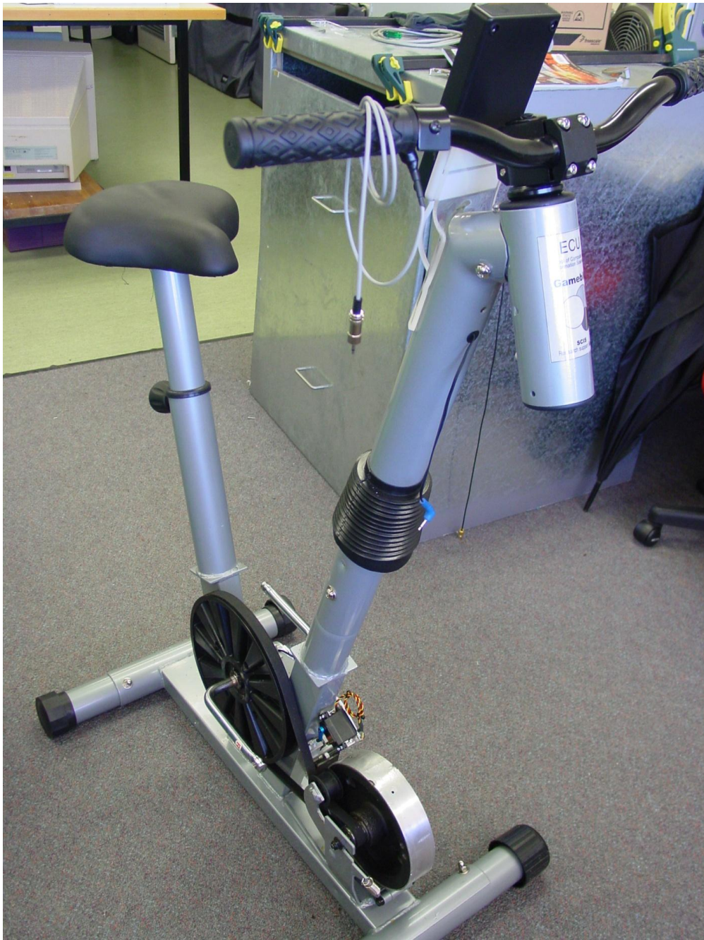
Figure 25 Modified Gamebike with the plastic cowlings, pedals and game control pad removed.
