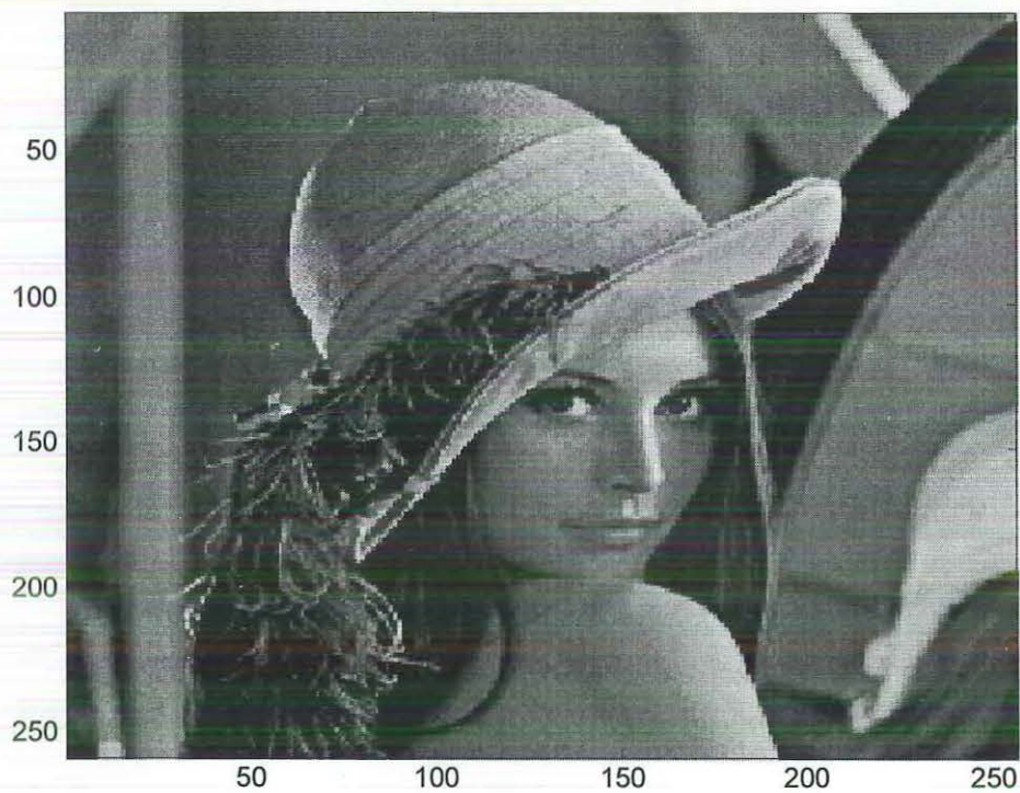
Embedded Image of Lenna PSNR of 42.40 dB and 2.32 bpp
