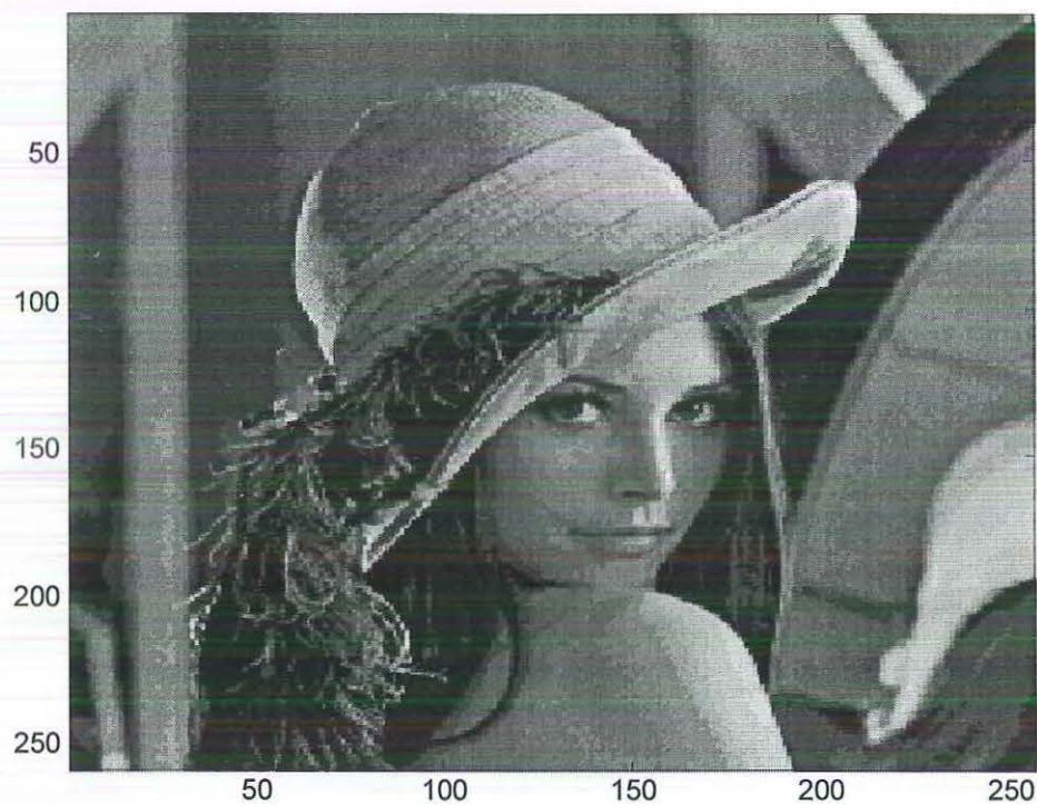
Figure 6.4 – Lossy Image of Lenna PSNR of 35.03 dB and 2.0 bpp.
