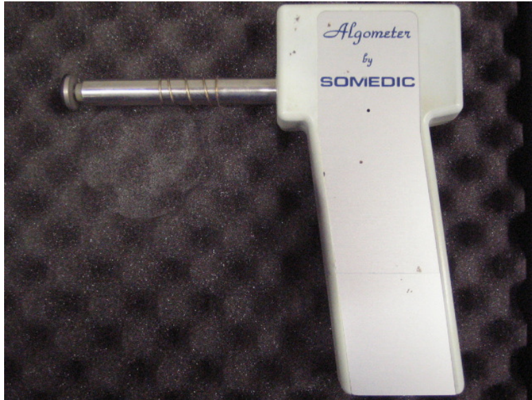
Figure 4: An algometer to assess PPT
