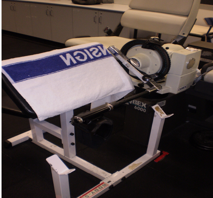
Figure 3: Cybex isokinetic dynamometer set-up with a preacher curl bench
