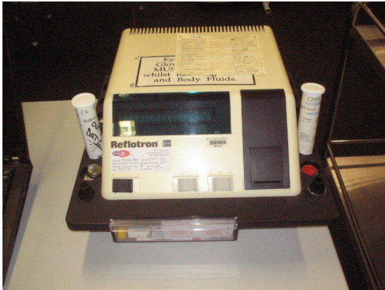
Figure 5: Reflotron to assess plasma CK activity
