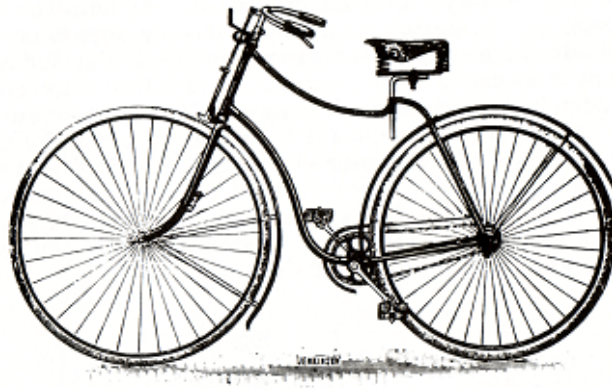
Figure 1. The first version of the safety bicycle (In Wilson, 1988, p. 221).
