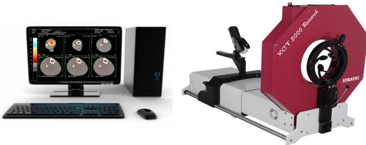
Figure 24. A pQCT machine with tibial measurement, knee brace and foot holder attachments (right) and the operating system with analysis software package (left).
