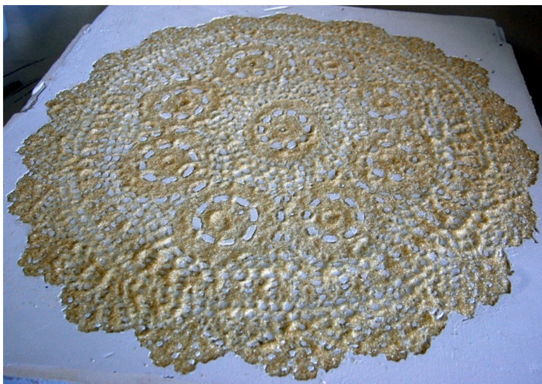
Figure 21: Lace mould for feast , date, made from plaster and silica packed with pâte de verre , ready to be fired, ECU studios, Mt Lawley.
