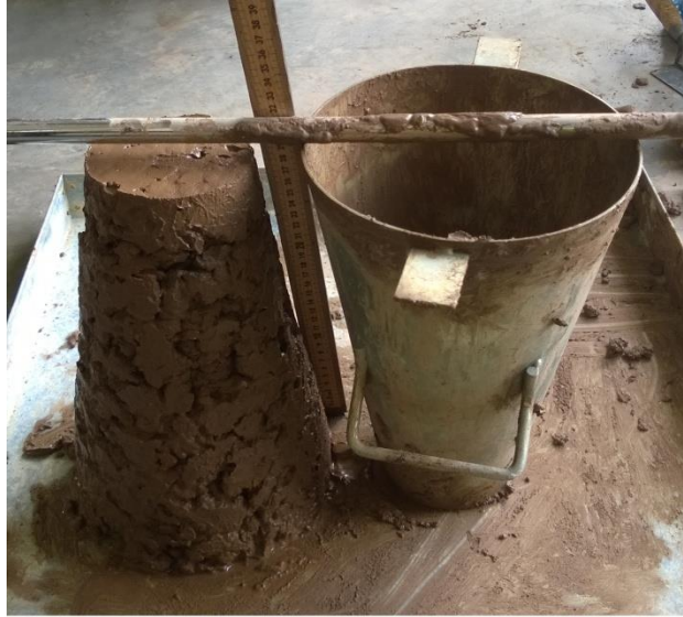
Figure 8.4: Determination of the slump of a fresh concrete.
