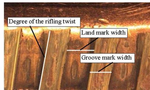
Fig. 5 Characteristics measurement on 2D image
