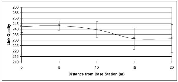
Figure 6: Change in Sun SPOT CORR level with increasing distance from base station.
