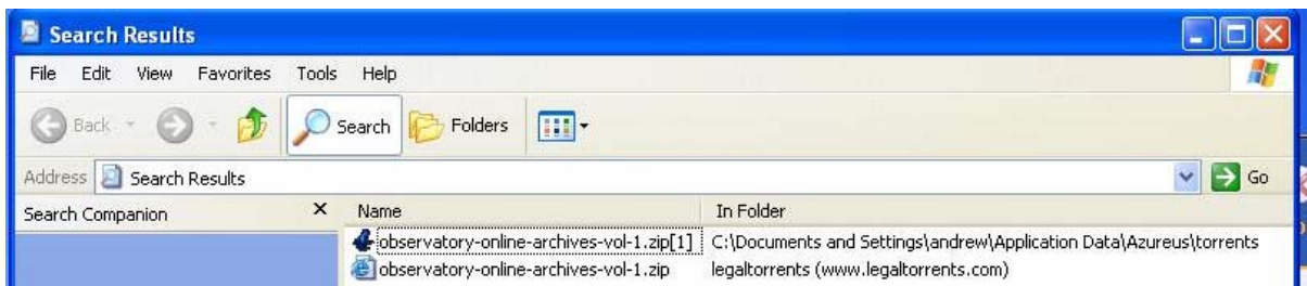
Figure 7: The erasure program P2PDoctor also left both the name of the file, and the web site from where the file was obtained in the Application Data folder
