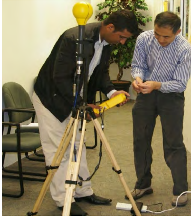
Figure 3.1: Irfan Ullah (L) and Dr Xiaoli Zhao (R) measuring RF-EME levels for the Telstra WCDMA 850 and 3GIS WCDMA2100 inside Building 21 at ECU using a selective radiation meter 3006.
