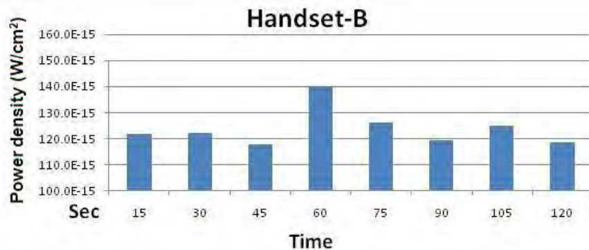
Figure 4.4: Radiation level measured for 2 min in Handset-B during standby mode.
