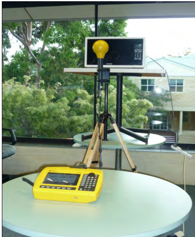
Figure 4.8: Microwave oven radiation power density measurements using selective radiation meter 3006.
