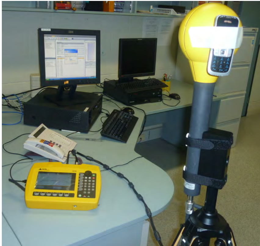
Figure 4.2: Selective radiation meter measuring mobile handset radiation level in standby, transmission and receiving mode
