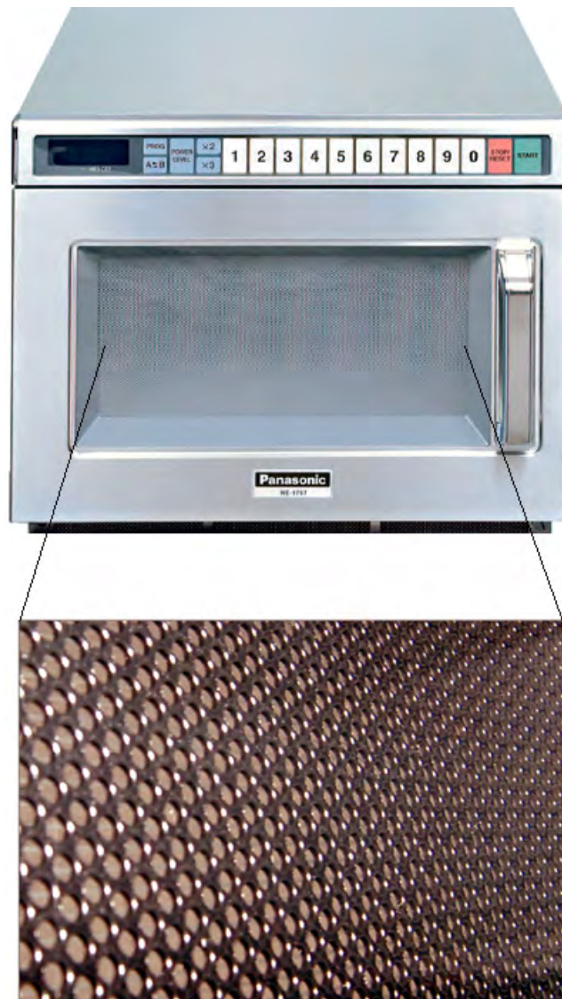
Figure 5.7: The metallic mesh of microwave oven door that exhibit high-pass filtering property to reflect microwave energy while transmit visual light for inside view [36]
