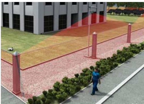
(c) Laser scanning across a perimeter
