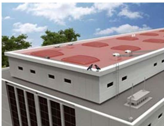
(e) Laser scanning for a high level roof protection against intrusion
