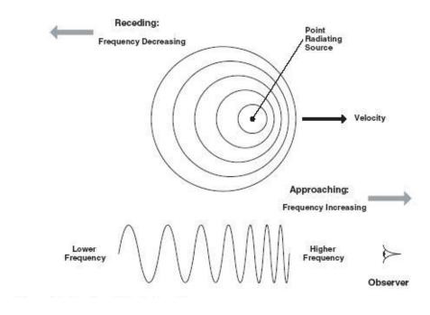
Fig. 2.6 – Doppler effect due to motion ("Aircraft Radar Basic Principle", n.d., Figure 3.7)
