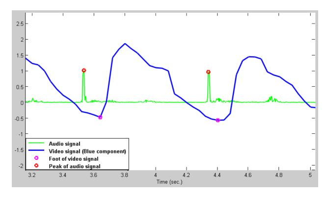
Fig. 5.5 – Results of peak and foot detection on an audio and video signal using Peakdet
