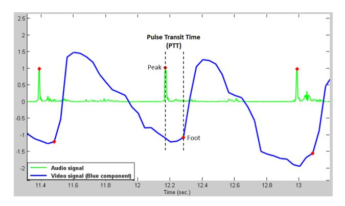
Fig. 5.3 – Peak-to-Foot measurement technique for PTT
