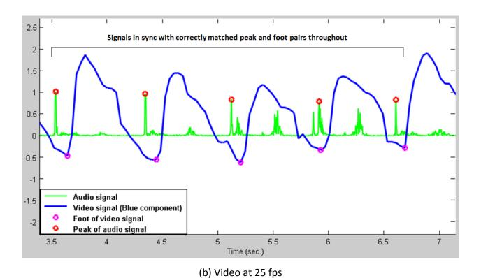
Fig. 5.6 – Audio/video waveforms for PWV with two different video frame rates
