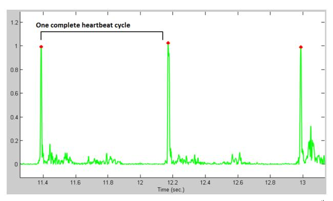
Fig. 4.9 – Audio waveform of a section of a heartbeat recording after being passed through a 6<sup>th</sup> order Butterworth band-pass filter and Hilbert transform
