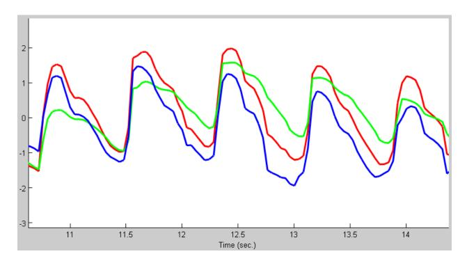
Fig. 4.2 – Section of a processed video signal showing the individual RGB channel data
