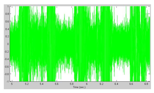
(b) A noisy and distorted signal at high recording volume
