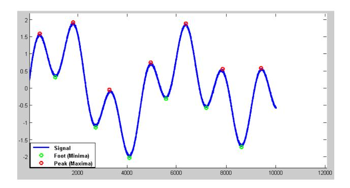
Fig. 5.4 – Sample peak detection in MATLAB using Peakdet
