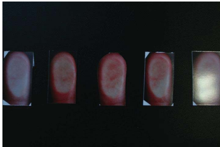
Figure 6 Artificial 2-dimensional depressed fingerprints
