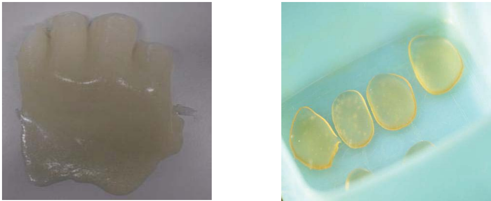
Figure 7 Replicated 3-dimensional back-of-hand and fingerprint overlays
