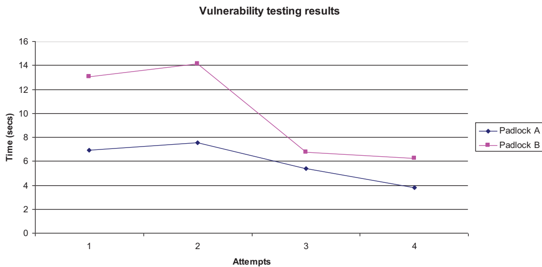
Graph 5: Vulnerability testing results (Sample sets)
