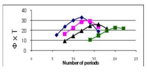
comparison with the typical size of a single nanocrystallite), reducing the total number of layers used provides additional technological benefits. The parameter  $T\times^{-}$ , where T is the transmittance of the MPC at the design wavelength and is the Faraday rotation angle at the same wavelength is found to be quite useful for comparing the efficiencies of different MPC designs.
