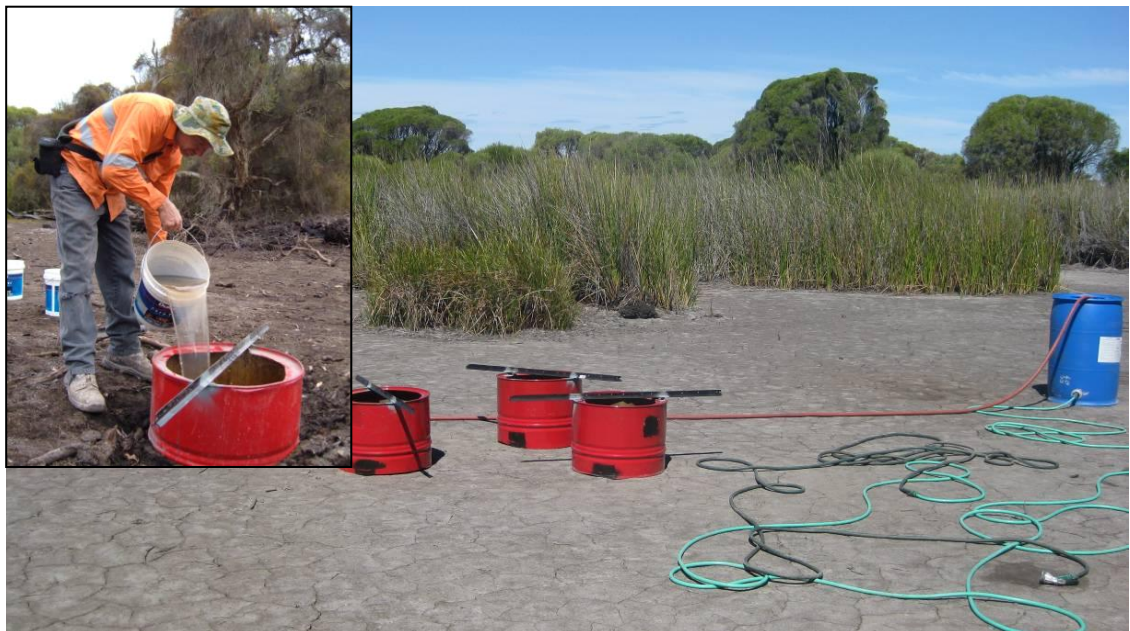
Plate 4. Half drums waiting to be used in EPP5. Large drum (on right) was filled from a water truck 100 m away and used for buckets to fill the drums (inset).
