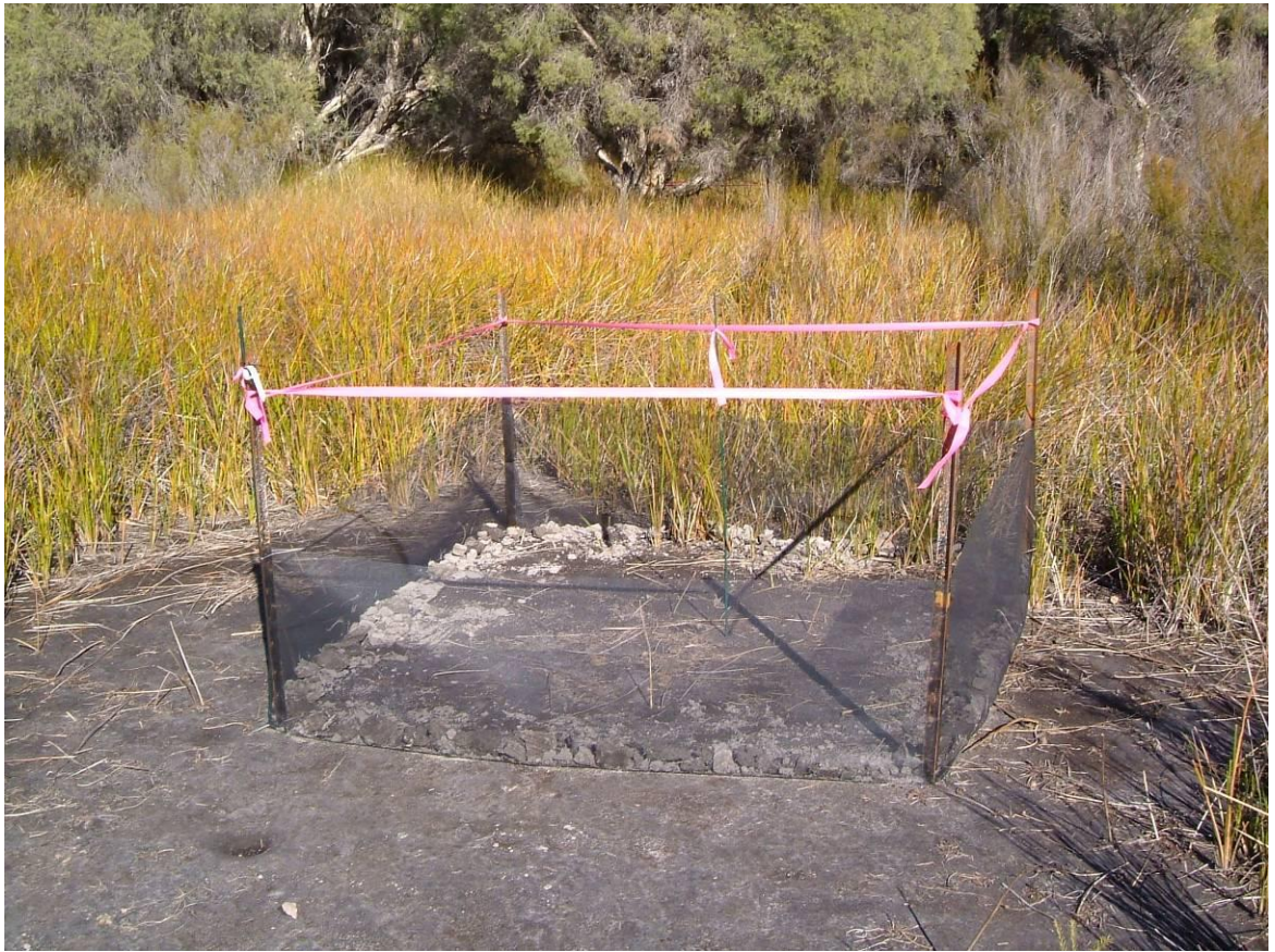
Plate 5. Vegetated lentocorral in EPP6. Flagging tape was to ward off animals, to prevent injuries to the animals and damage to the enclosure.
