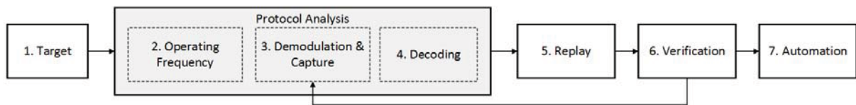
Figure 1. RF Replay Attack Methodology
