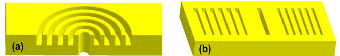
Fig. 1. Schematics of a plasmonic structure composed of a subwavelength aperture flanked by surface corrugations. (a) Three-dimensional bull's eye structure. (b) Two-dimensional slit-grating structure.
