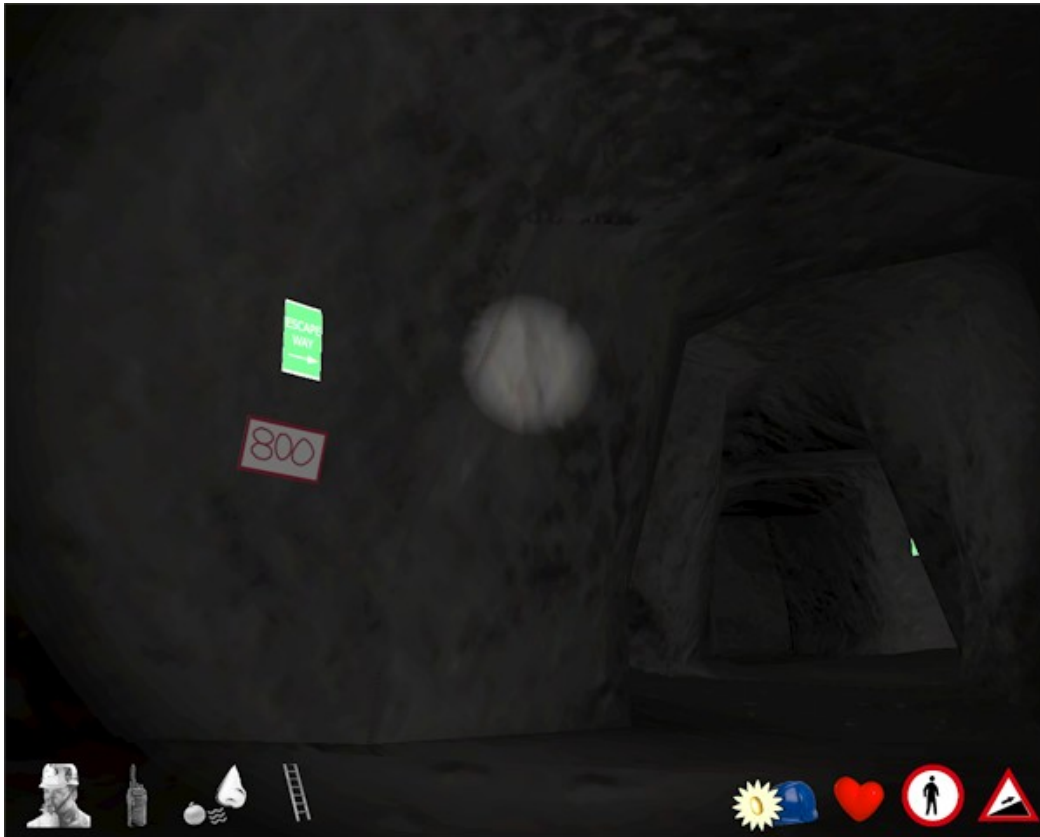
Figure 5.10. Application of emissive properties to approximate the reflective properties of escape rise signs
