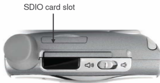
Figure 8 – Top down view of SD/SDIO slot on Treo 650 7
