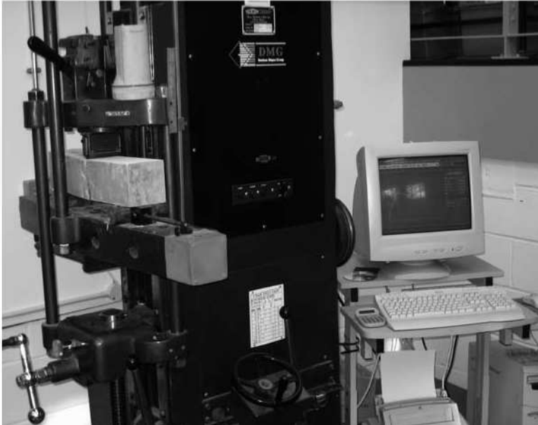
Figure 6 – Denison [DMG 67], beam sample and linked computer.
