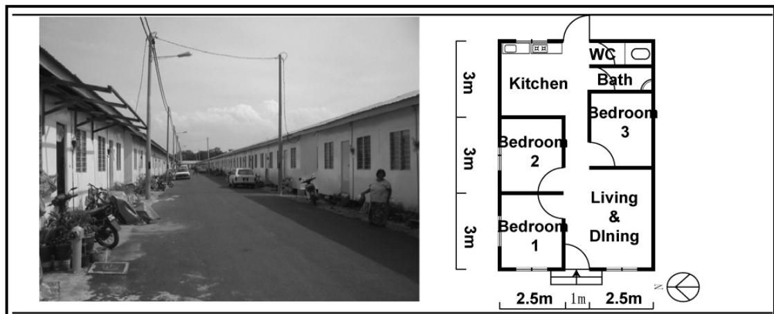
Fig. 4.1: Temporary Longhouses and Typical Floor Plans
