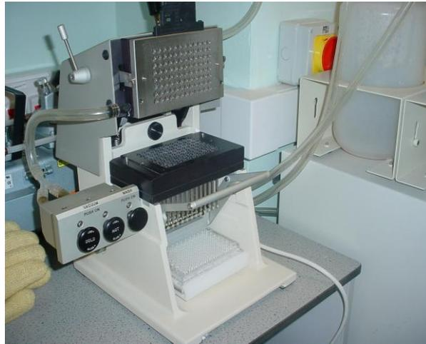
**Figure 3.13:** Packard Filter mate Harvester
