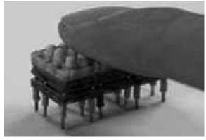
Fig. 4 ElectroActive Polymer Braille display by Ig Mo Koo
