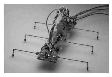
Fig. 3 Artifical mosquito with muscle-wires (Micronet Munich).
