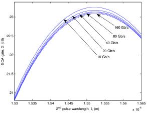
Figure 4: SOA gain profile of the second input pulse against the wavelength at different input data rates.
