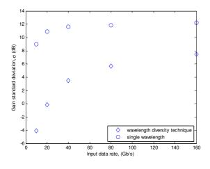
Figure 5: Gain standard deviation against input data rates for single wavelength and wavelength diversity technique.
