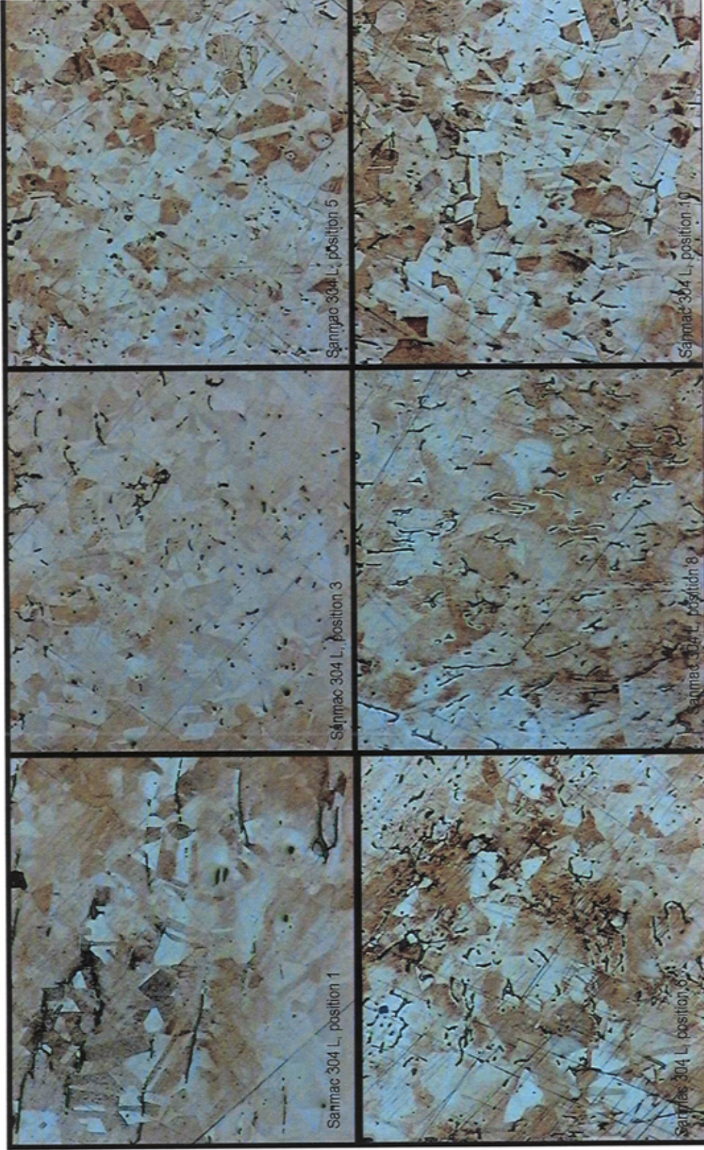
Figure 29 Stainless Steel, Magnification 50X, Etch agent: concentrated hydrochloric acid
