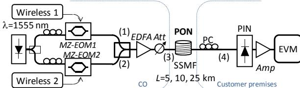
Figure 2. Experimental set-up for converged MB-OFDM UWB and WiMAX IEEE 802.16e transmission performance analysis over PON.
