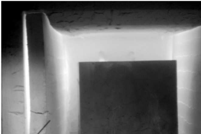
Figure 4 – Concrete cube in 1000°C furnace
