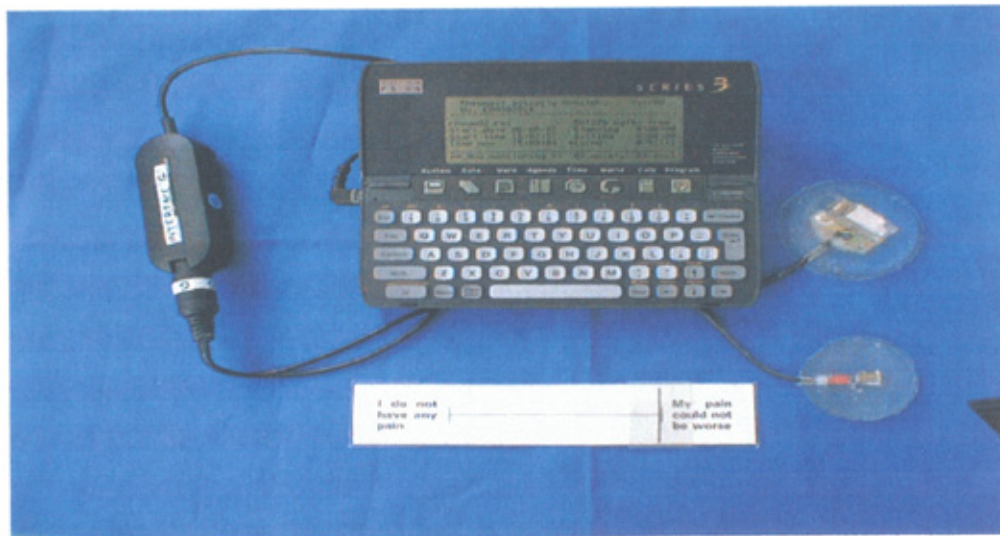
Figure 4.5 NUMACT ambulatory monitoring equipment
