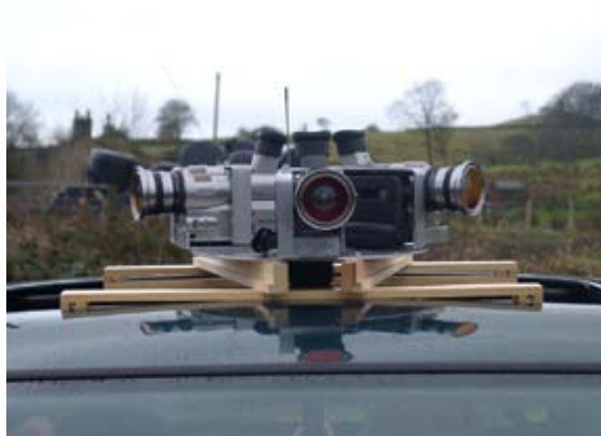
Fig. 57 Vehicle mounted tripod with three digital video cameras with wide-angle lenses
