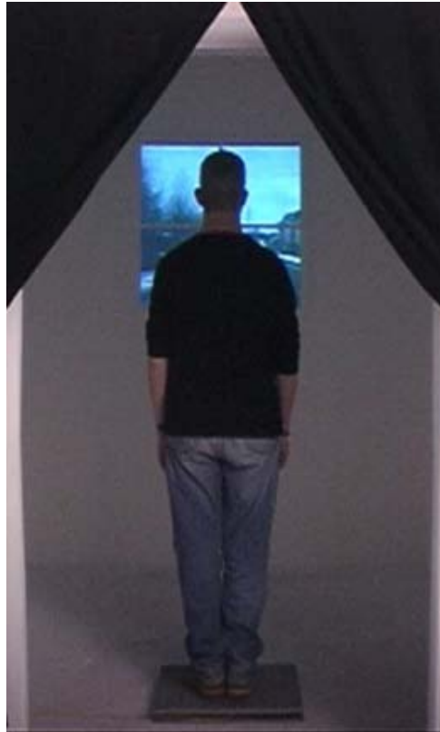
Fig. 64 Subject and force plate inside Kansas
