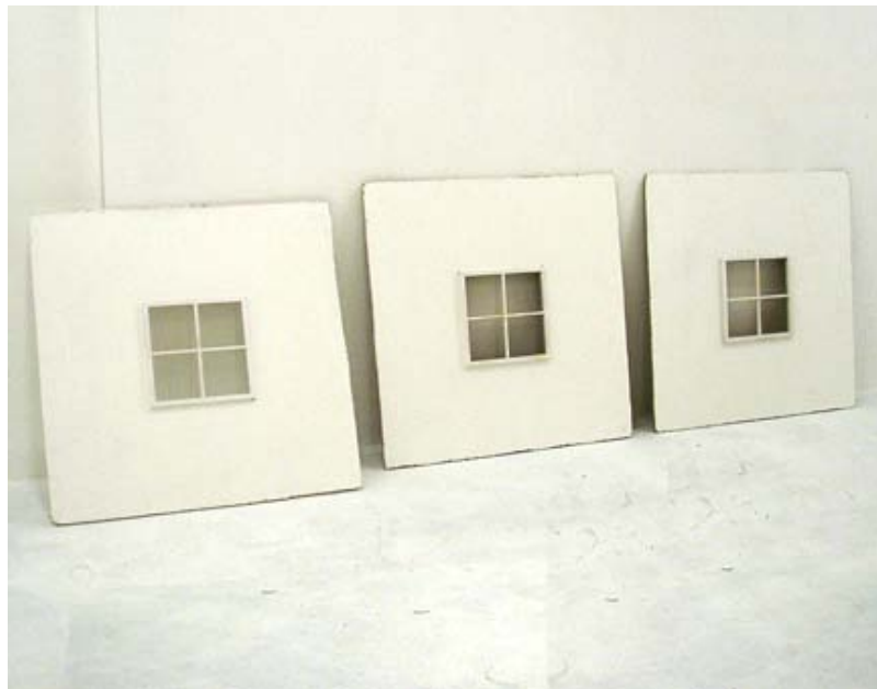
Fig. 67 Interchangeable small aperture inserts (The outside frame is equal in size to the opening for the larger apertures shown in Fig. 66)
