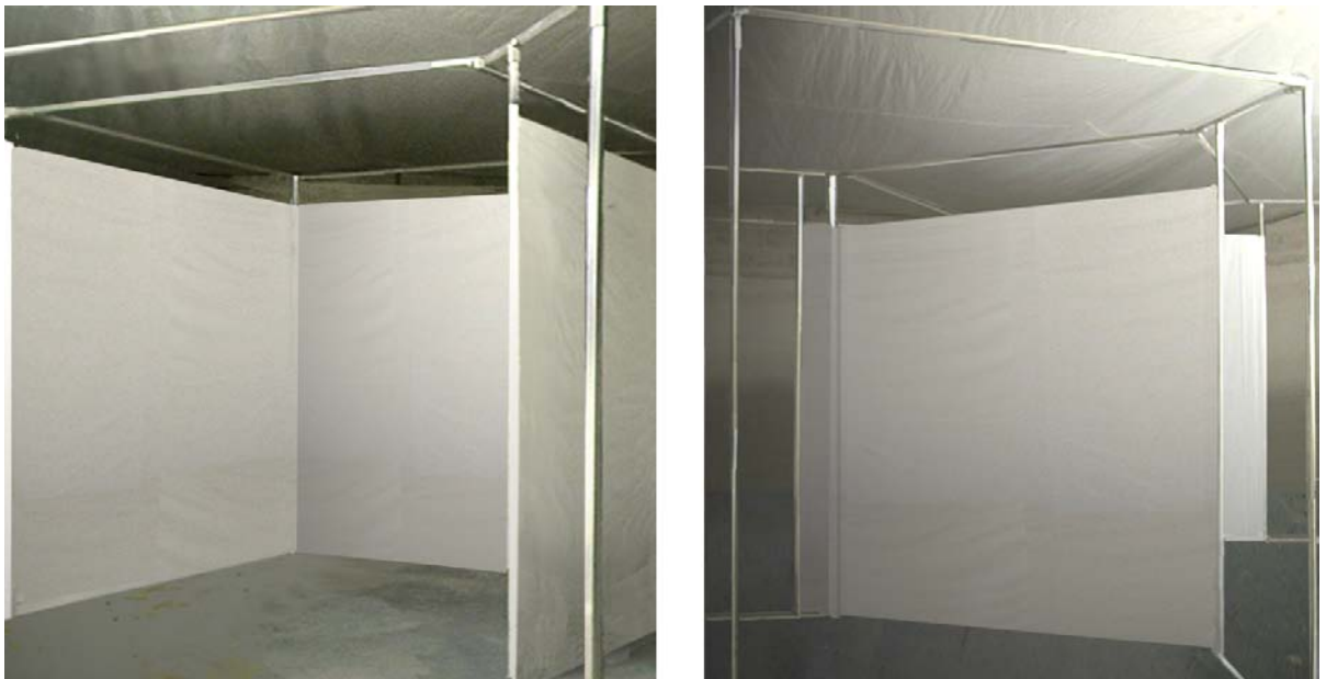
Fig. 34 MIE2: Full scale aluminium framework with three rear projection screens
