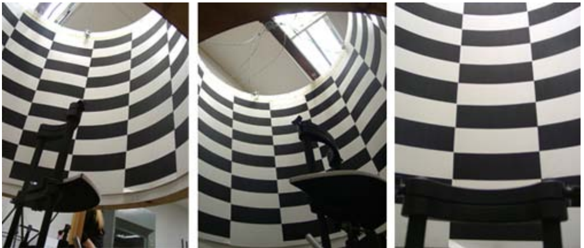
Fig. 42 Optokinetic drum (interior view) Laboratory of Dr Fred Bonato, Kings College, New Jersey, US
