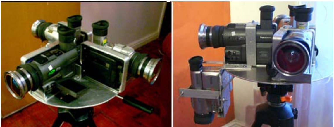
Fig. 6: Three and four camera configurations with floor standing tripods
