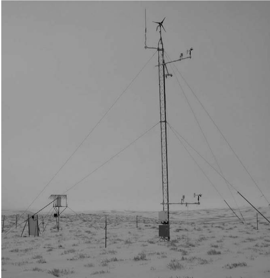
FIG. 3. Michigan River meteorological tower and shielded precipitation gauge located at 2600 m MSL. in the North Park MSA, near Walden, Colorado. Stakes shown in the photograph held wire for an electric fence to protect the site from livestock and elk herds frequenting the area.
