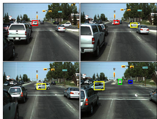
图 3 Intersection 运动障碍检测 Fig. 3 Moving obstacles detection intersection sequences
