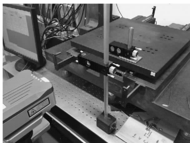
(b) Y轴沿Z轴旋转误差(偏摆误差)的测量 (b) Measurement of rotation error(deflection error) for Y axis along Z axis
