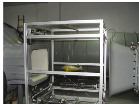
Fig.5 WDPSS-8 suspension system in wind tunnel.
