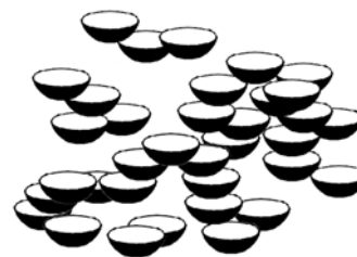
Figure 33 The nematic structure of bowlic molecules as an imitation of that of disk-like molecules.
