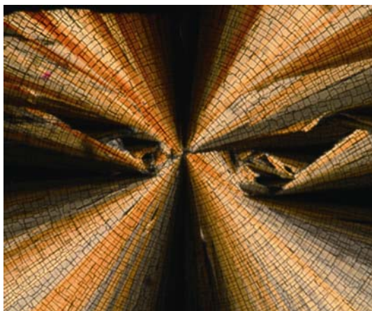
Figure 21 The POM photograph of point disclination with s = +1 ( \delta = 0^\circ ) decorated by lamellae presented in the mosaic-like morphologies of the CTV-2 sample. The scale is 100 \mu\text{m} , and the director distribution map is shown on the right side.
