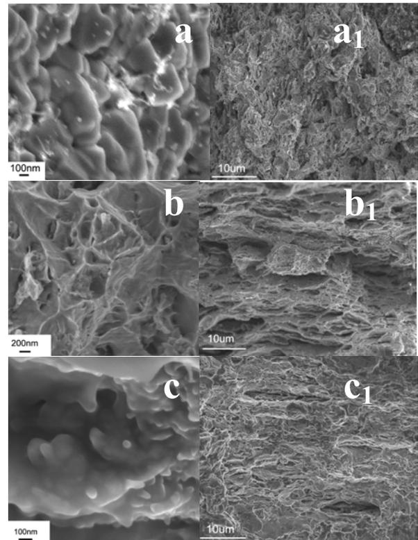
**Fig. 2** SEM of the fracture surfaces MWCNTs/Cu composites (1 wt % of MWCNTs). (a),(a1) Vacuum hot pressing. (b), (b1) hot rolling, (c), (c1) annealing after hot rolling.
