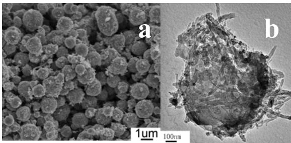
**Fig. 1** (a) SEM image of the MWCNT/Cu<sub>2</sub>O composite spheres. (b) TEM image of the MWCNT/Cu<sub>2</sub>O
