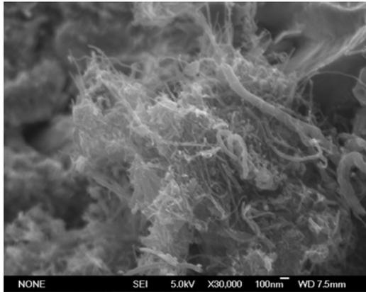
**Fig.3** SEM of the fracture surfaces of MWCNTs/Cu composite (mechanically mixing)
