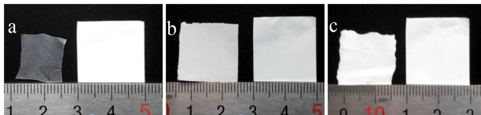
Fig. 3. Dimensions of separators before and after subjected to heat treatment at 150 °C for 30 min (a) pristine PE separator; (b) ST coating separator; (c) SP coating separator.
