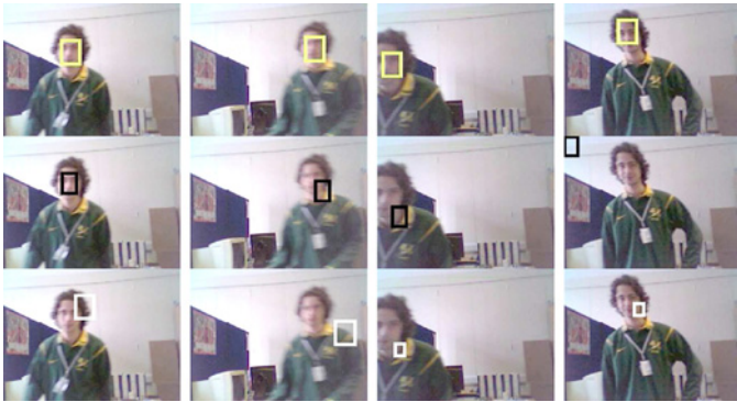
Fig. 4. Face sequence 1. Tracking results of the proposed tracker (top row); standard mean shift tracker (middle) and particle filtering (bottom row). Frames 26, 56, 318, and 432 are shown. The video size is 320 \times 240 and the frame rate is 10 frames per second (f/s).
