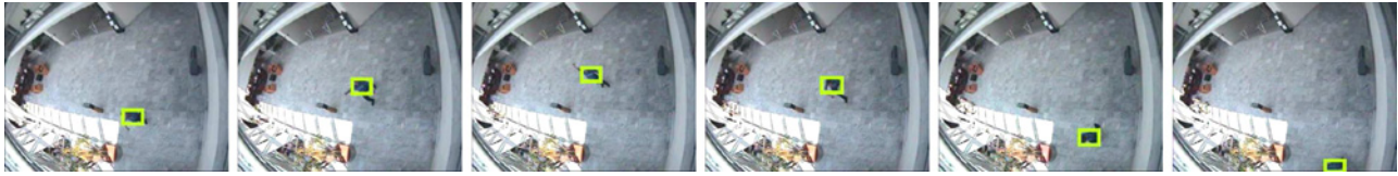
Fig. 6. Walker sequence 1. Tracking results of the proposed generalized kernel tracker. Frames 20, 40, 60, 90, 115, and 130 are shown. The video size is 384 \times 288 and the frame rate is 25 f/s.
