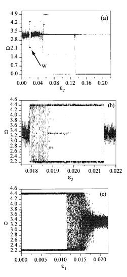
FIG. 2. Phase phenomenon among the global signals. (a)  $\varepsilon_2$  versus the average frequencies  $\Omega$ , with  $\varepsilon_1=0$ . Region *w* corresponds to the two clusters of the PS phenomenon. The step size is  $\Delta \varepsilon_2 = 0.5 \times 10^{-3}$ . (b) An enlargement of region *w* with  $\Delta \varepsilon_2 = 0.5 \times 10^{-4}$ . (c)  $\varepsilon_1$  versus  $\Omega$  with  $\varepsilon_2 = 0.021$  and  $\Delta \varepsilon_1 = 0.5 \times 10^{-4}$ .
