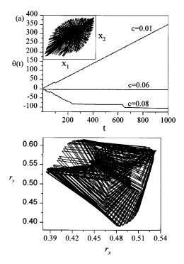
FIG. 3. Plots of simulation results with two one-way coupled map lattices. (a) The inner plot shows one of the attractors on the  $x_1-x_2$  plane while the outer plot is phase difference  $\theta(t)$  versus time *t* at different values of coupled strength. (b) The trajectories on the  $r_x - r_y$  plane with c = 0.06.
