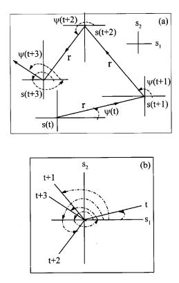
FIG. 1. The mechanism caused by the proposed phase definition. (a)  $\psi(t)$ ,  $\psi(t+1)$ ,  $\psi(t+2)$ , and  $\psi(t+3)$  are the phase states of the points s(t), s(t+1), s(t+2), and s(t+3) on the  $s_1-s_2$ plane while *r* is the distance between two points. (b) All the phase states are considered at a specific direction (counterclockwise) with respect to the origin.
