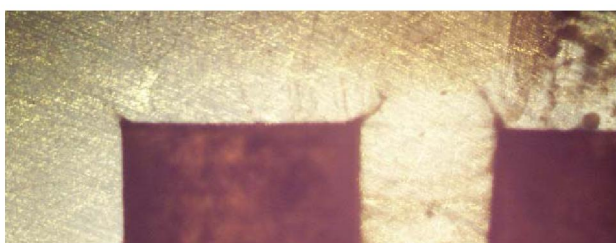
Figure 4 Nanofibers bundles at the vertex of the collector. The electrospinning voltage (between spinneret and collector) is 12kV, with electrode-to-collector distance of 11cm. Collection time: 30s; The polymer solution used is 7.32%PEO.
