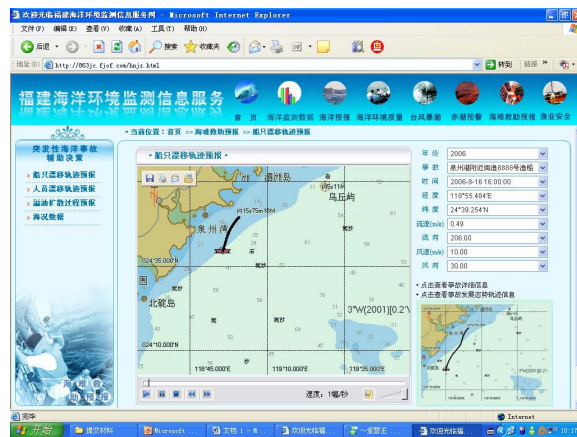
Figure 6. A numerical computation simulation based oil spilling forecasting result in Taiwan Strait example is released on web.
